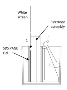
**Figure 2.** Insertion procedure for the 8x10cm or 10x10cm gel white screen into the *XCell SureLock® Mini-Cell tank* (image courtesy of *Life Technologies*).
