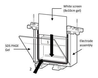
**Figure 3.** Insertion procedure for the 8x10cm gel white screen into the *Bio-Rad mini-PROTEAN* tank (image courtesy of *Bio-Rad*).
